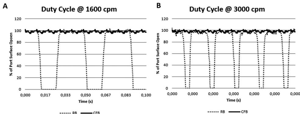
**Fig. 2.** Duty cycle of RB (dotted line) and CFB (continuous line) defined as percent of open port surface over the cutting cycle at 1,600 cpm (A) and 3,000 cpm (B). Because of the invariant port surface available for aspiration, CFB duty cycle is the same in Positions A–C, and is consistently close to 100%.
